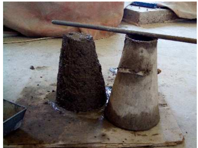
Figure 2. Measurement of workability of concrete.
