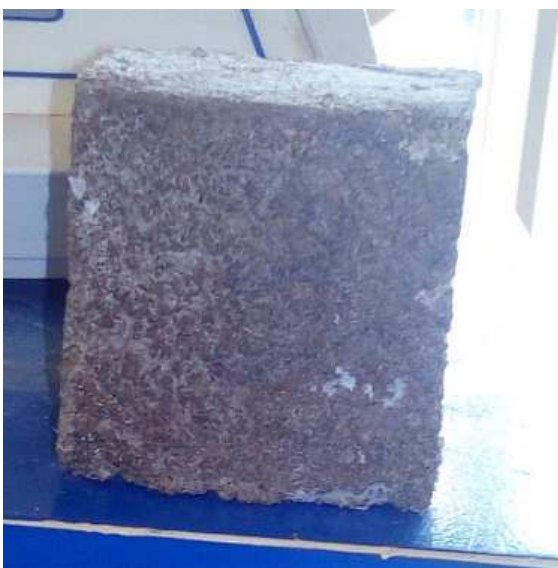
Figure 1. Sample for Strength Activity Index test.
